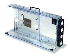
The BWT-100™ is a portable benchtop wind tunnel for thermal characterization of components, boards and heat sinks. The unit is made of Plexiglas™, weighs less than 8 pounds (4 kg) and produces flows up to 400 ft/min (2 m/s). It can be operated horizontally or vertically to adapt to direction-sensitive electronic cooling systems.
