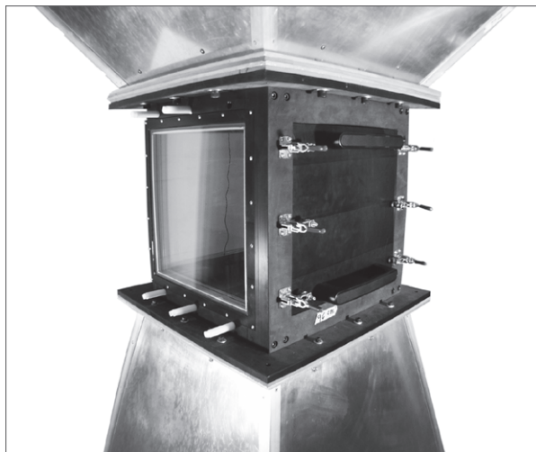
Close-up view of the CLWT-100's test section
