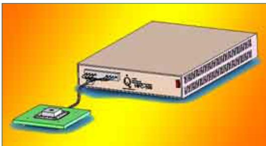
Illustration of the HFC-100 Heat Flux Controller with simulated chip capable of dissipating 1 kW of heat over 1 cm<sup>2</sup>.
