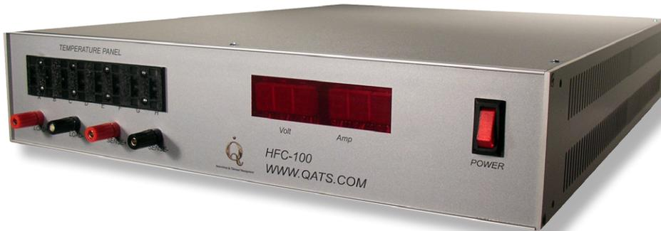
The Heat Flux Controller™ is a high heat flux chip simulator capable of measuring and controlling the amount of heat in a resistive element. The HFC-100™ comes with a chip simulator capable of dissipating 1k /cm<sup>2</sup>. The design of the heater block insures minimal heat loss to the ambient, hence a more accurate thermal resistance determination of either heat sinks or cold plates.
