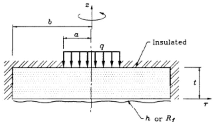
Figure 2. Heat Source on a Heat Sink Base [2]
