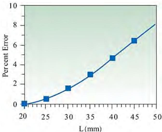
Figure 4. Percent Error Between the Analytical and the Approximate Solution of Spreading Resistance for the Example Shown in Figure 3 [3]
