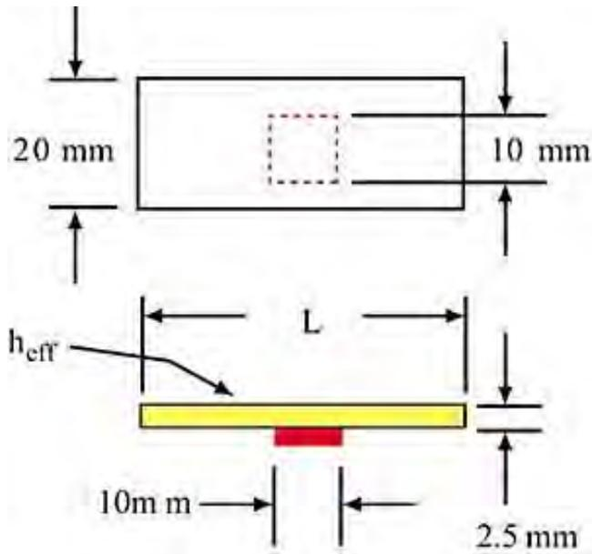
Figure 3. Example Problem For Comparing Analytical and Approximate Solutions for Spreading Resistance [3]
