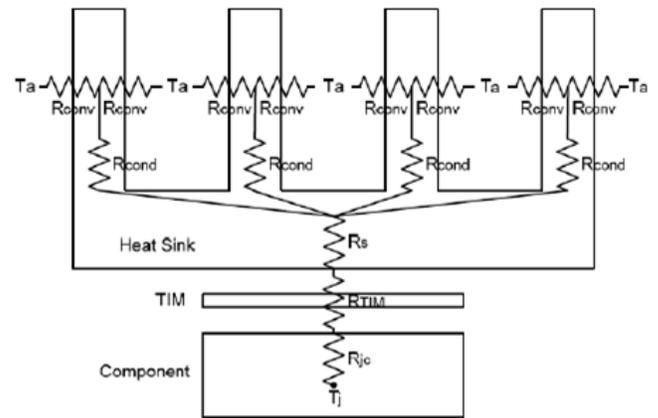
Figure 1. Resistance Network of a Typical Heat Sink in Electronics cooling [1]
