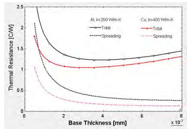
Figure 5. Total and Spreading Resistance of the Example Shown in Table 1 for a 50 mm Heat Sink
