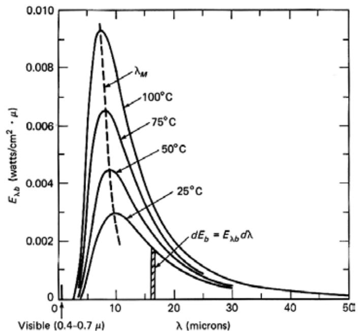
Figure 1. Low Temperature Spectral Distribution of Emissive Power [2].
