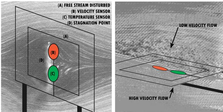
Figure 6. Effect of Large Sensors in Flow Dispersion.
