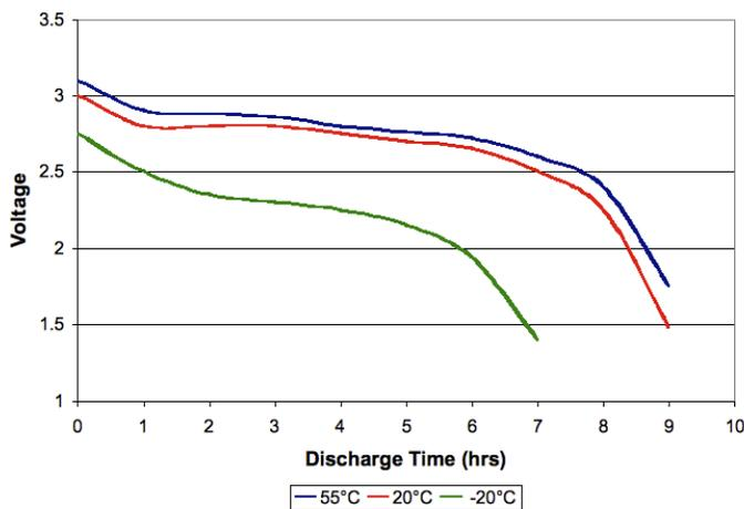
Figure 2. Discharging Performance of a Sample Lithium-Ion Battery Pack as a Function of Temperature [3].
