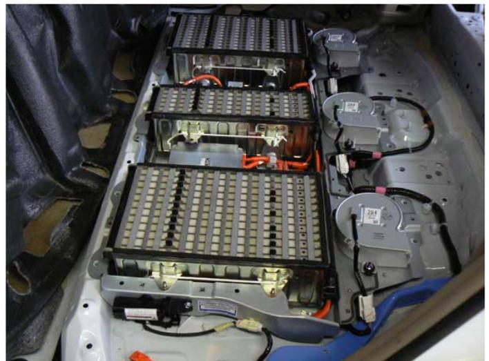
*Figure 1. Location and Orientation of the Toyota Highlander Hybrid Battery Pack [1].*
