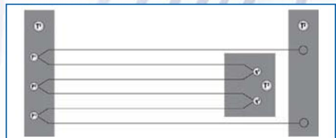
Figure 3. Series-connected thermocouples forming a thermopile.
