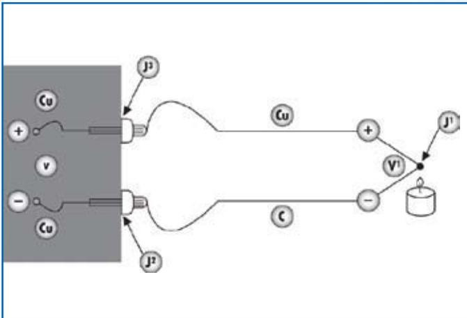
Figure 1. Measuring junction voltage with a DMV [1].
