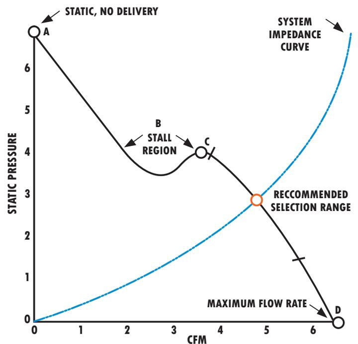
Figure 1. Typical Overlay of a System Curve and Fan Curve.
