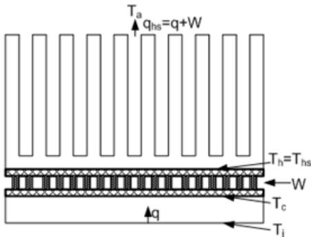
Figure 3. Schematic of a Heat Sink with TEC
