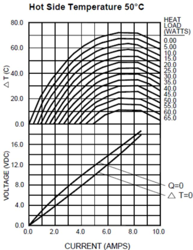
Figure 6. Marlow RC12-8 TEC Performance Curves [2]
