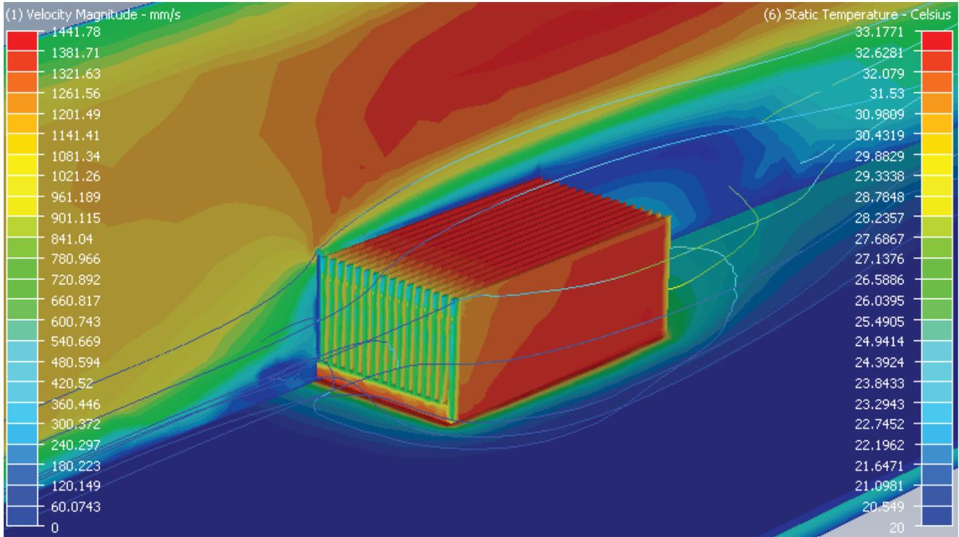
Figure 5. CFD Image of a Straight Fin Heat Sink in an Unducted Environment, Dissipating 10 W at an Inlet Air Flow Velocity of 1 m/s (~200 LFM).
