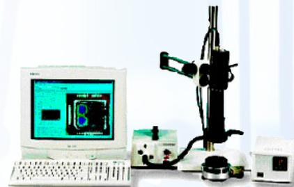
**Figure 8. The Thermview™ System for Macro and Microscopic (Down to 1µm) Surface Temperature Measurement [4].**
