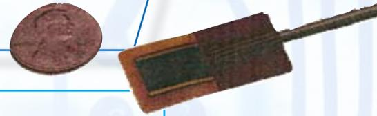
Figure 1. Surface-Mounted RTD
