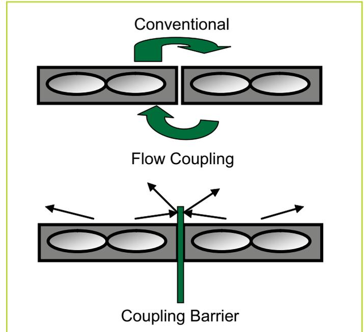
Figure 5. Parallel Fan Flow Coupling and Respective Remedy [3].
