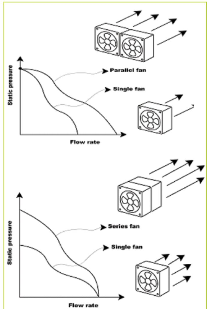
Figure 3. P-Q Curve for Fans in Parallel (3a) and in Series (3b) [4].
