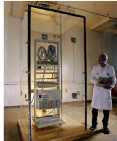
*Figure 1 - Environmentally Controlled Chamber for NEBS Testing [1]*
