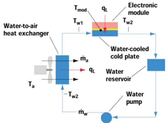
Figure 1. Closed Loop Liquid Cooling System [1].
