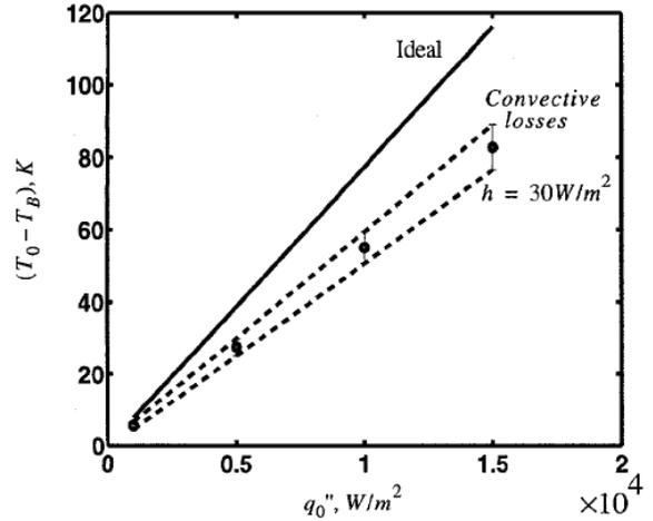
Figure 8. Gardon Gauge Calibration [3].
