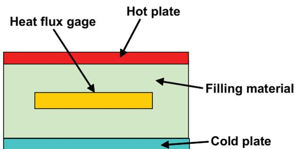
Figure 4. Calibration of a Heat Flux Gauge Using Hot and Cold Plates [1].
