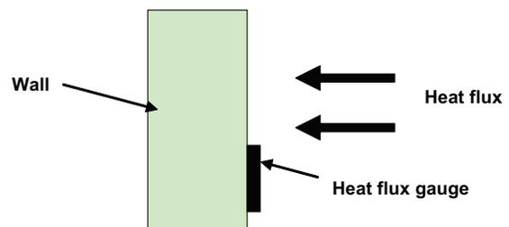
Figure 2. Heat Flux Gauge for Measuring Conductive Heat Flux
