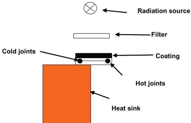
Figure 3. Radiation Sensor with Lateral Sensitivity [1].
