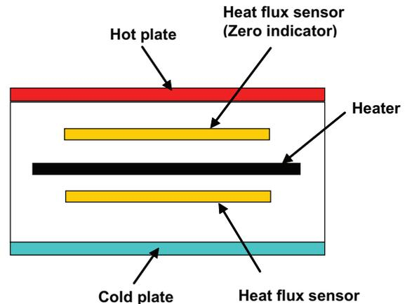
Figure 5. Calibration of a Heat Flux Gauge Using Hot and Cold Plates and a Heater [1].
