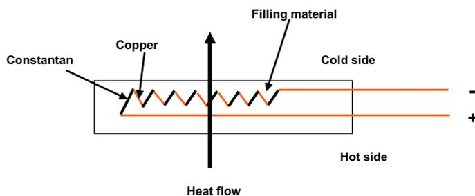
Figure 1. Thermopile Concept of a Heat Flux Sensor Based on Thermocouples in Series.
