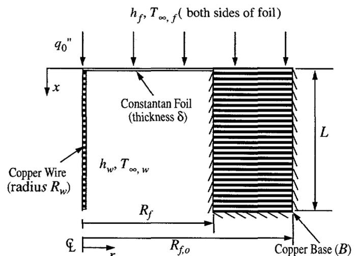
Figure 6. Model of a Gardon Gauge [3].
