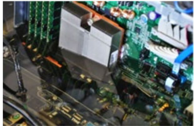
Figure 2. A Server Motherboard Being Immersed in Liquid Coolant in A Server Rack [1]
