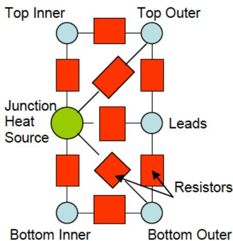
Temperatures averaged. Nodes communicate with each other. Surface nodes with environment, internals may have a heat source associated with them
