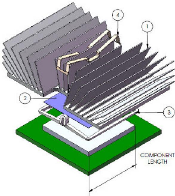
Figure 3 - maxiFLOW/superGRIP™ Heat Sink with Thermal Interface Material
