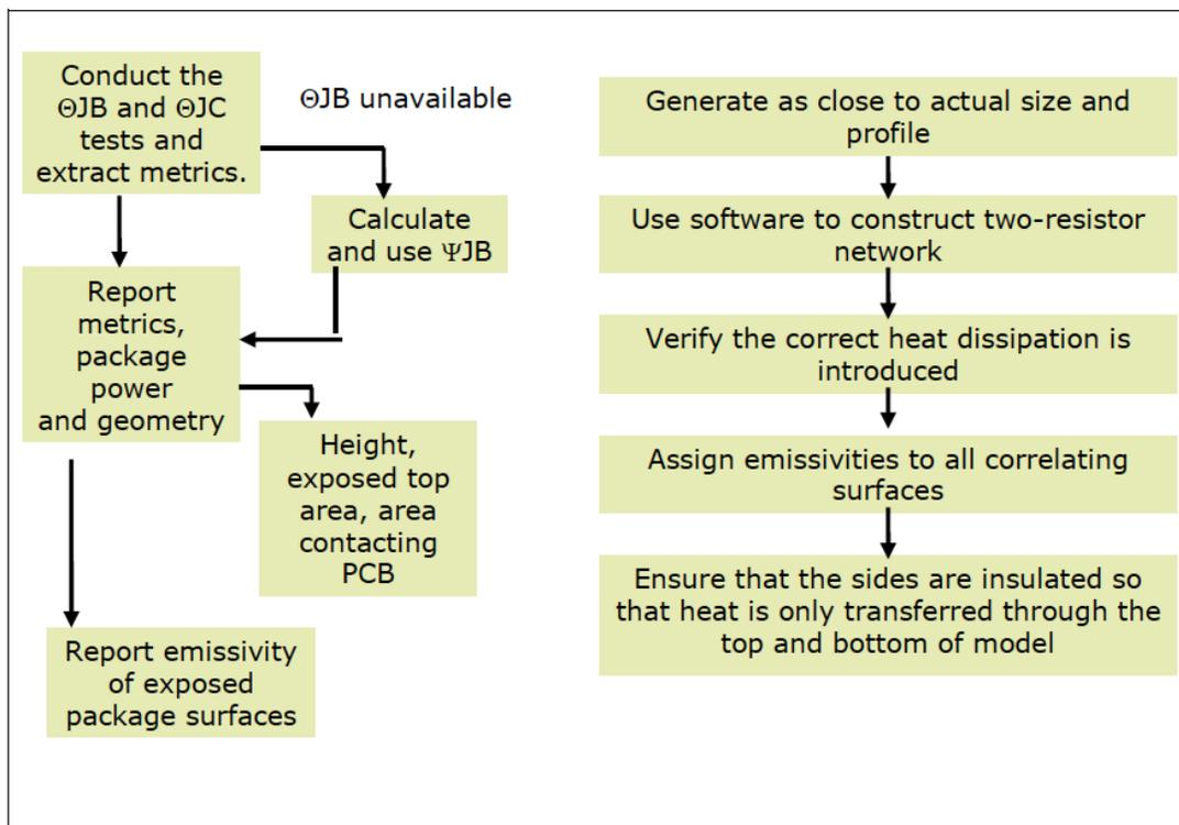
Table 2 - Thermal Network and 3D Simulation Methods
