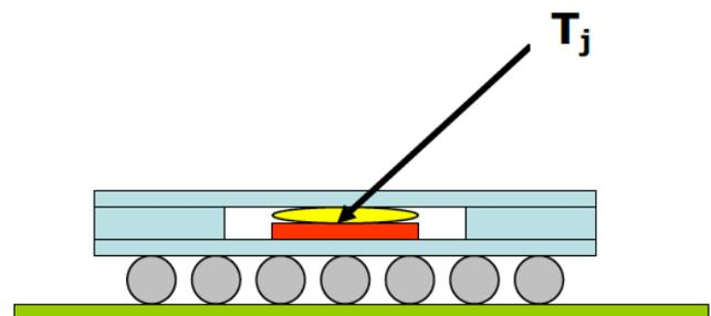
Figure 1 – Package Attached to PCB via BGA
