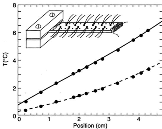
Figure 3. Data Obtained by Measuring the In-Plane Thermal Conductivity,  $k$  of a Sample of Printed Wiring Board with Many Vias [2].
