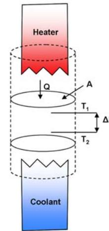
Figure 1. Typical Thermal Conductivity Measurement Diagram [1].
