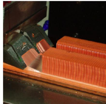
*Figure 7.- Typical Image of Skived Heat Sink [12], [13]*
