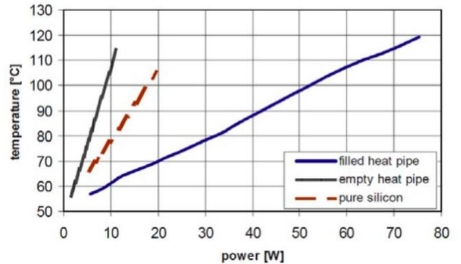
Figure 6. Maximum Temperature on the Dissipative Component Depending on the Input Power [1].
