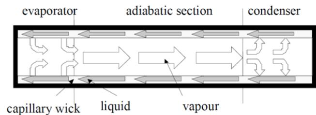
Figure 1. Operating Principle of a Heat Pipe [1].
