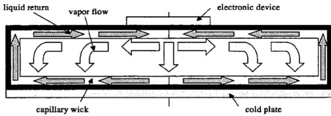
Figure 2. Operating Principle of a Flat Heat Pipe being used as a Heat Spreader [3].
