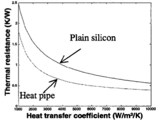
Figure 3. Comparison of the Thermal Resistance of a Heat Pipe vs. Plain Copper (a) and vs. Plain Silicon. Each Comparison features the Same Dimensions between the Heat Pipe and the Plain Solid Material [3].
