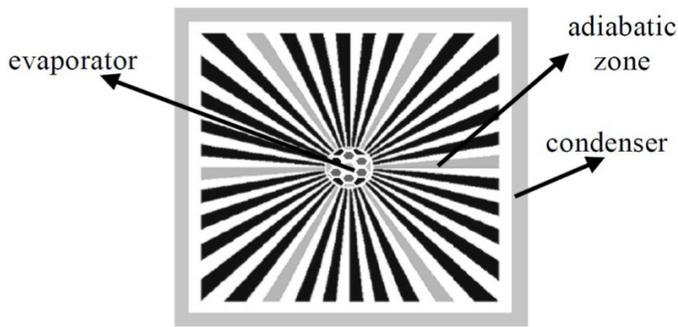
Figure 5. Capillary Wick Design of the Heat Pipe [1]
