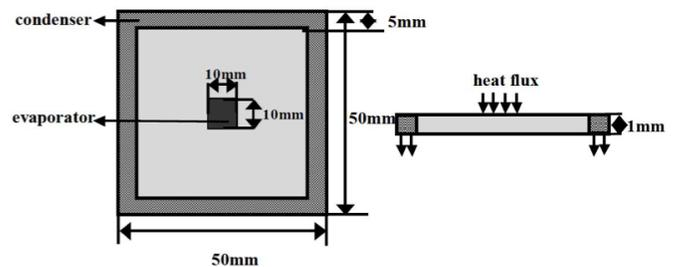
Figure 4. Silicon Heat Pipe Design [1].
