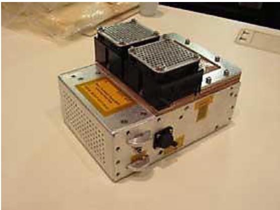
*Figure 2. A Test Unit Containing Heat Pipes and a Data Acquisition System Used to Study the Processes of Fluid Dynamics in the Microgravity Conditions Aboard the International Space Station. [6]*
