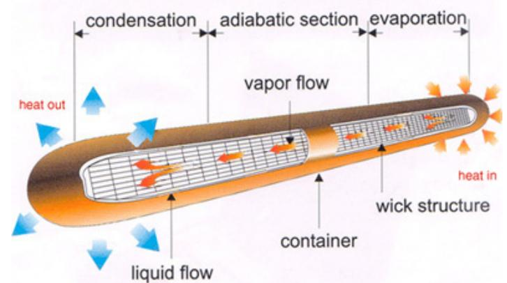
*Figure 1. Figure 1: Heat in a Heat Pipe is Absorbed by Liquid at One End. The Liquid Becomes Hot Vapor which Flows to the Cold End where It Condenses and Releases the Latent Heat. The Re-condensed Liquid Flows Back to the Hot End. [2]*
