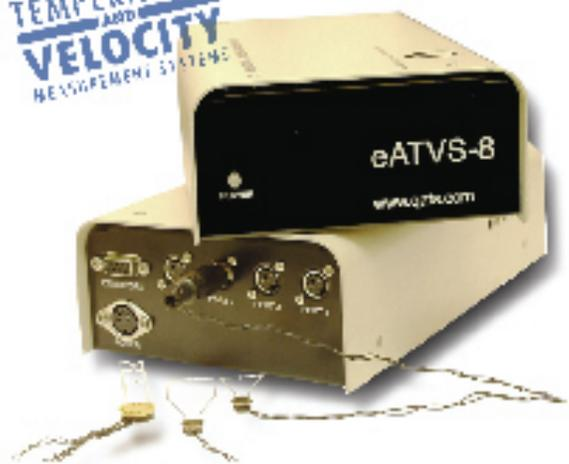
ATS' Automatic Temperature and Velocity Measurement Systems deliver unmatched accurate, stable and versatile performance for all aspects of thermal analysis. Fully automated, these research-quality instruments take accurate single- or multi-point measurements of air temperature, velocity and surface temperature in complex environments, such as PCBs and electronics enclosures.
