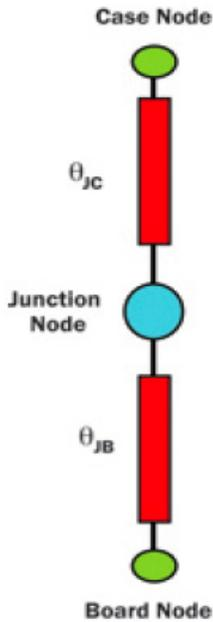
Figure 1. A Two-Resistor Compact Thermal Model [1].
