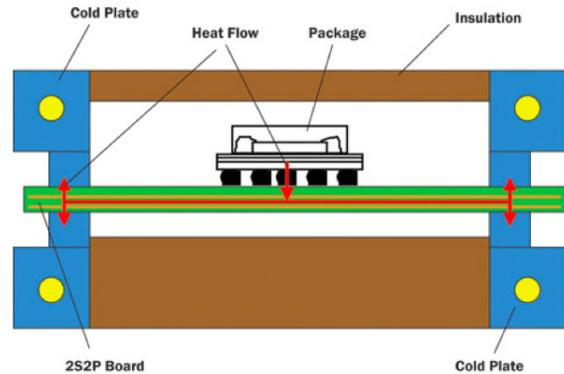
Figure 2. Fixture for Measuring  $\theta_{ja}$  [1].
