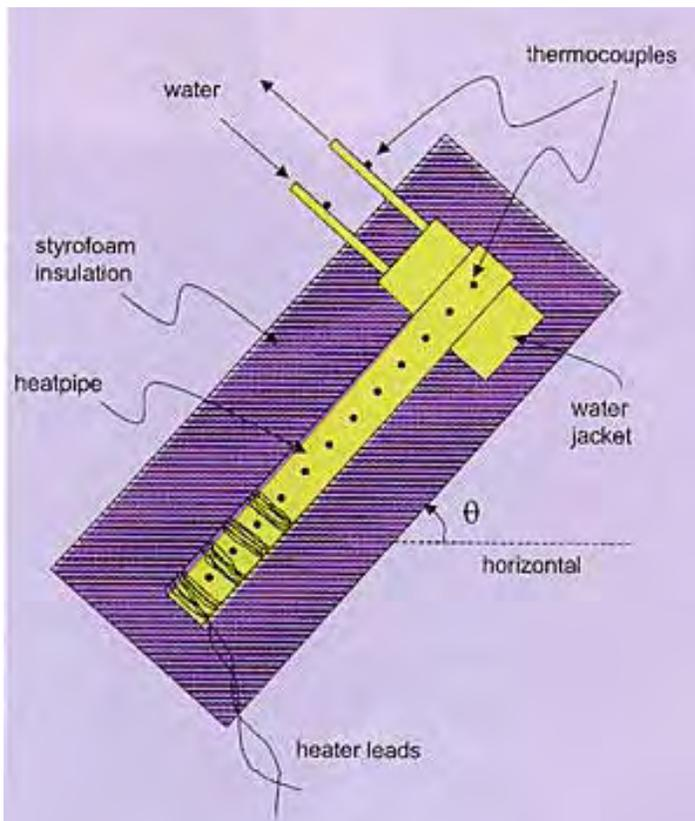
Figure 4. Test Setup Used in the Experiment 2 [3]
