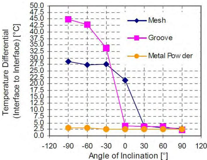
Figure 7. Thermal Performance of 4 mm OD, 200 mm Length Heat Pipes at Different Inclination Angles, for Heat Load 5 W [2]
