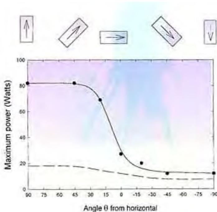
Figure 11. Thermal Performance of a 6.35 mm OD, 300 mm Length Sintered Copper Powder Wick Heat Pipe at Different Inclination Angles, for 95 °C Operating Temperature [3]
