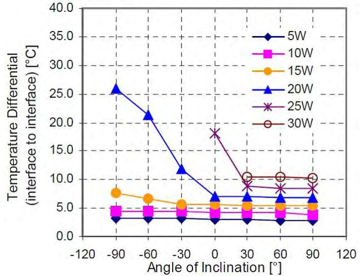
Figure 8. Thermal Performance of a 6 mm OD, 200 mm Length Sintered Powder Metal Heat Pipe at Different Inclination Angles, for 35 °C Operating Temperature [2]
