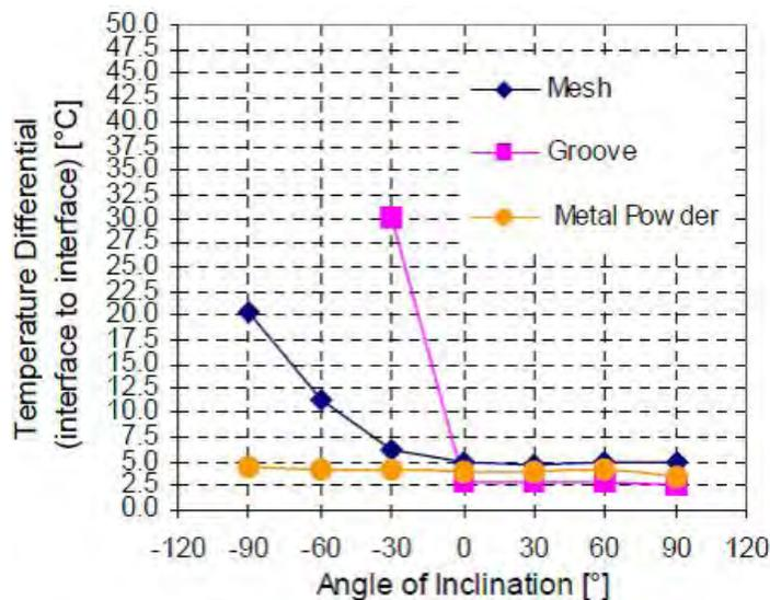
Figure 5. Thermal Performance of 6 mm OD, 200 mm Length Heat Pipes at Different Inclination Angles, for Heat Load 10 W [2]
