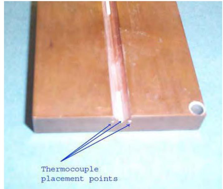
Figure 3. Thermocouples Location on the Evaporator and Condenser Blocks [2]
