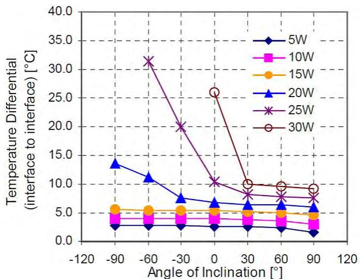
Figure 9. Thermal Performance of a 6 mm OD, 200 mm Length Sintered Powder Metal Heat Pipe at Different Inclination Angles, for 45 °C Operating Temperature [2]
