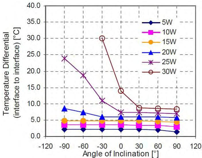
Figure 10. Thermal Performance of a 6 mm OD, 200 mm Length Sintered Powder Metal Heat Pipe at Different Inclination Angles, for 55 °C Operating Temperature [2]
