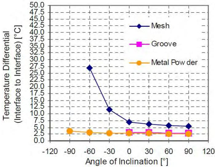
Figure 6. Thermal Performance of 5 mm OD, 200 mm Length Heat Pipes at Different Inclination Angles, for Heat Load 10 W [2]
