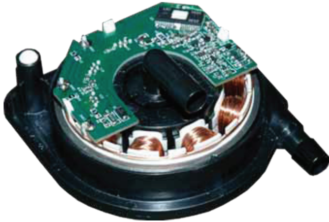
Figure 5. Intel Integrated Liquid Cooling Loop [3].
