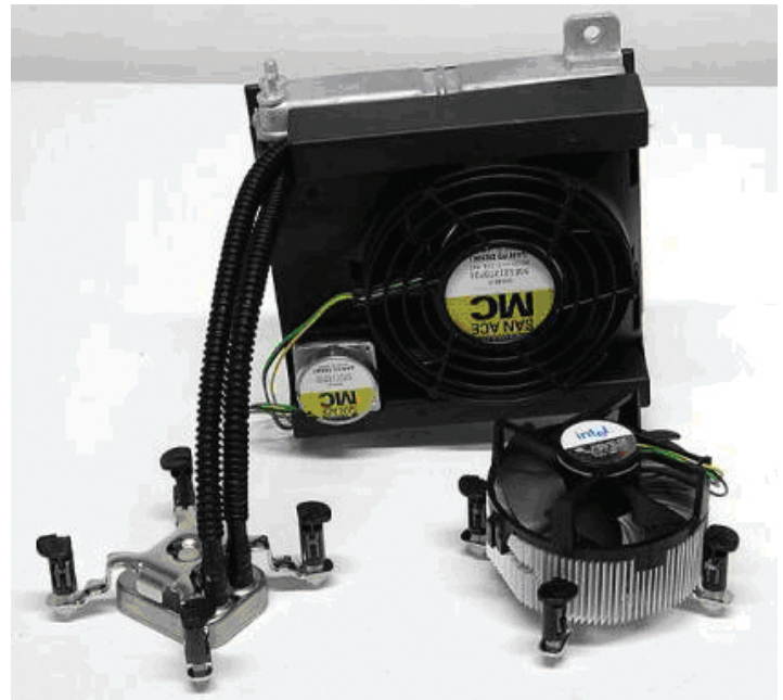
Figure 3. Integrated Forced Liquid Cooling System Compared to an Air Cooled Solution [2].
