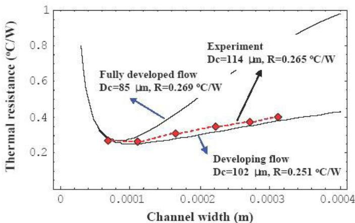
Figure 4. Microchannel Heat Exchanger Performance vs. Channel Width [3]
