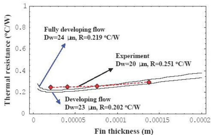
Figure 5. Microchannel Heat Exchanger Performance vs. Fin Thickness [3]
