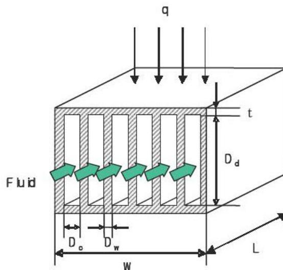
Figure 3. Geometry of a Microchannel Heat Exchanger [3]
