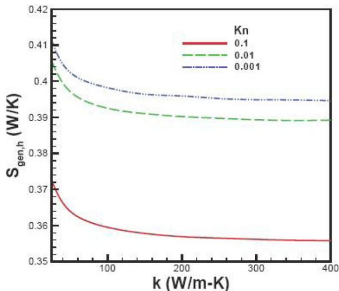
Figure 7. Entropy Generation as a Function of Heat Exchanger Material [4]
