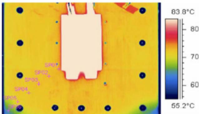
Figure 8. Temperature Distribution of Vapor Chamber Surface [6]
