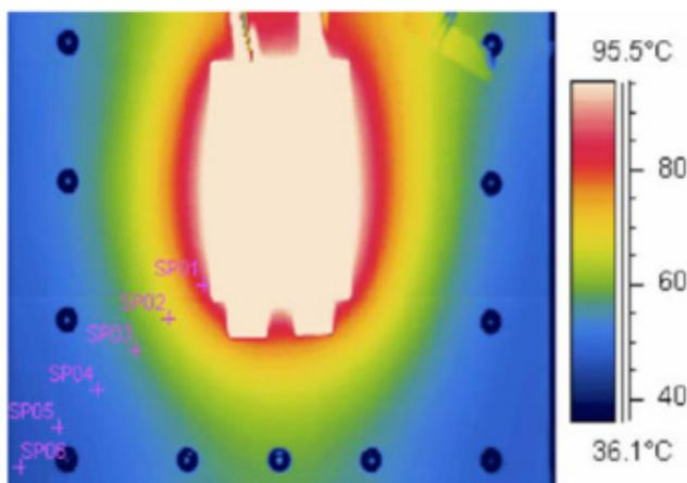
Figure 9. Temperature Distribution of Copper Heat Spreader Surface [6]
