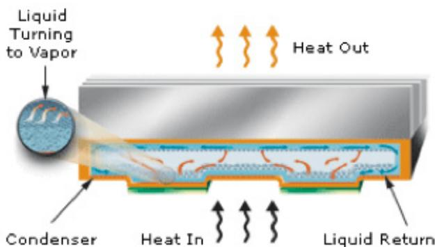
Figure 1. Vapor Chamber [4]
