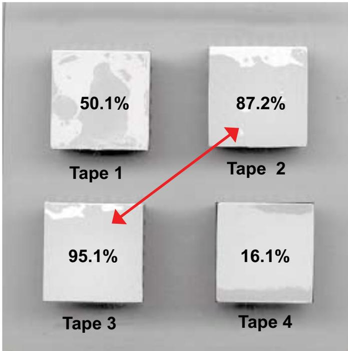
Figure 1. Picture of Contact Area as a Function of Tape Thickness (Tape1 = 0.005", Tape 2 = 0.010", Tape 3 = 0.015"). Dark areas show adhesive wetout. [2].
