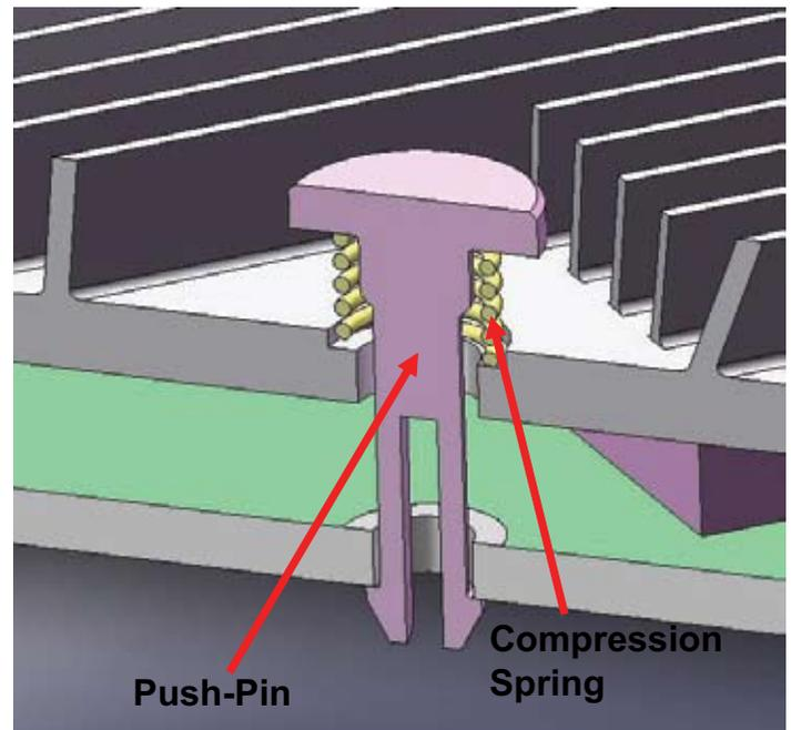
Figure 6. Cross Section View of Push-Pin & Compression Spring Attachment.
