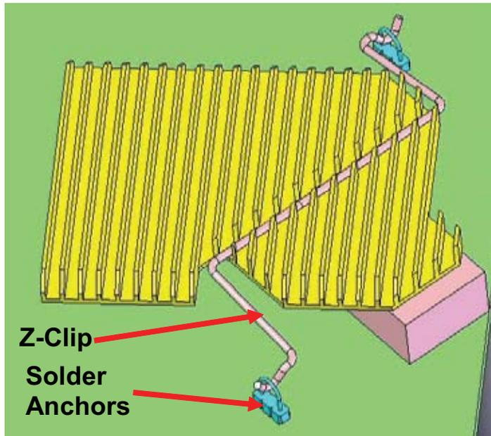
Figure 3. Heat Sink with Z-clip and Solder Anchors.
