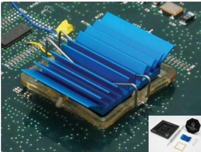
Figure 5- maxiGRIP™ Heat Sink Attachment Solution.
