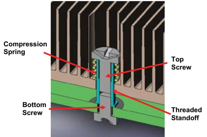
Figure 7. Cross Section View of Threaded Standoff with Compression Spring.
