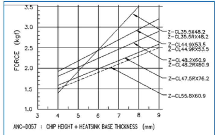
Figure 4. Typical Loads for Z-clips [3].
