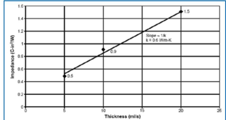
Figure 2. Graph of Tape Thermal Impedance with Respect to Tape Thickness.
