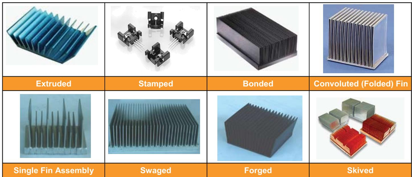
Figure 1. Heat Sinks Fabricated Using Different Manufacturing Processes [1].
