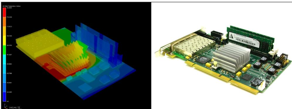
*Figure 4. CFD Simulation of the GE Fanuc Intelligent Platform's WANic Packet Processor PCI Card with the ATS-725 maxiFLOW™ Heat Sink Installed, Along Side a Sample Card.*
