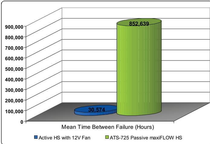
Figure 6. Comparison of Cooling Solutions for the GE Intelligent Platforms WANic 3860 Card In Terms of Mean Time Between Failures
