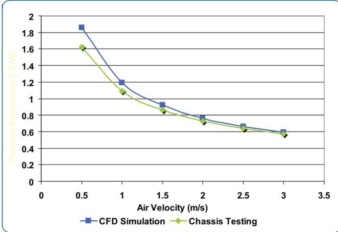
Figure 5. The Results of CFD Simulations and Chassis Testing of the ATS 725 maxiFLOW™ Heat Sink. GE Fanuc Recommends and Airflow of at least 275 LFM if a Passive Heat Sink is Used
