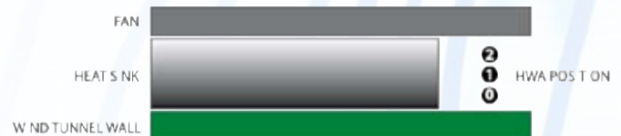
Figure 2. Side View of the Test Rig, Showing the Vertical Position of the Velocity Probe (HWA).
