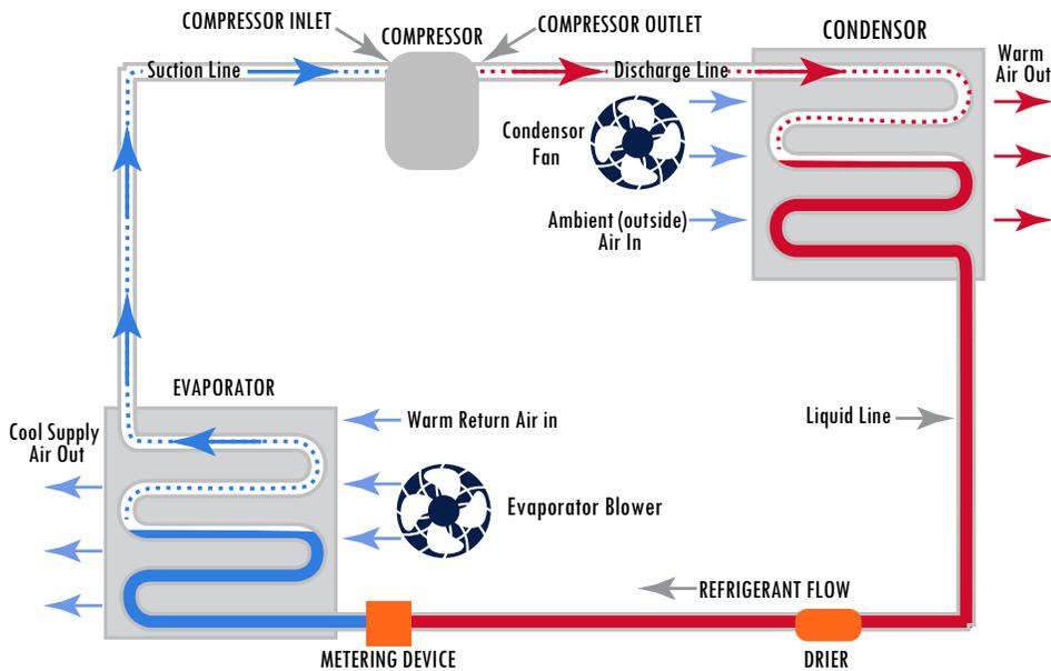
Fig. 1. The standard refrigeration cycle for recirculating chillers.
