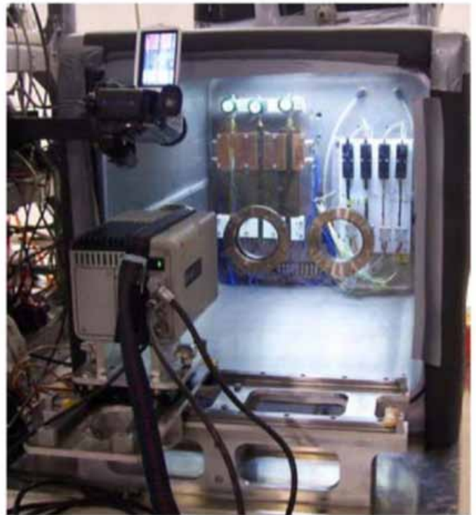
Figure 2. (a) Experimental Rack Onboard Airbus A300. (b) Vacuum Chamber with Heat Pipes. [4]
