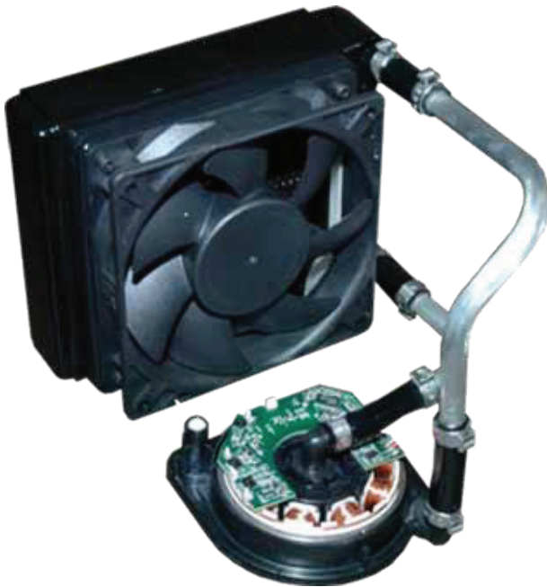
Figure 4. Intel's Integrated Cold Plate and Liquid Pump Assembly [3].
