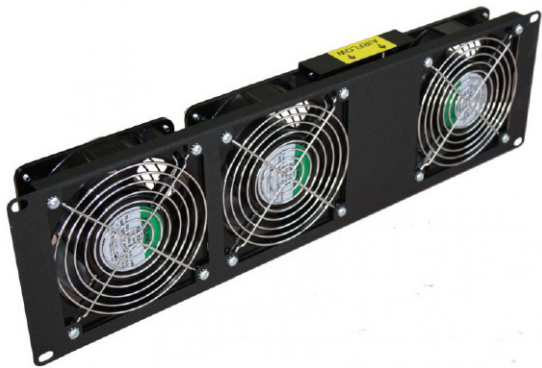
Figure 4. A rack mounted fan unit that provides 90 cubic feet of air per minute to cool hotspots in a server cabinet.
