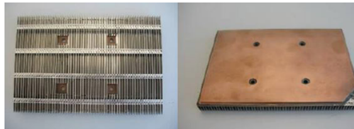
Figure 11. Heat sink with vapor chamber C-1. [7]
