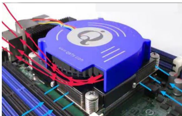
Figure 3. The QuadFlow CPU cooler draws air from four sides, passing it through cooling fins and expelling warm air. (Advanced Thermal Solutions, Inc.)
