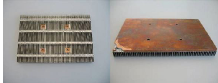
Figure 10. Heat sink with vapor chamber B-1. [7]
